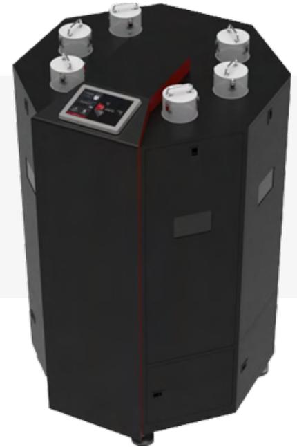
CVM(Clogged Vibration Method) powder feeder is new type of powder feeding system. It has impressively stable powder feed rate, perfect lifetime and broad feeding rate range, from 0.05g/min to 20g/min for single CVM Feeder block based on titanium. Applicable for gravity powder supply method and direct powder supply method with gas.
